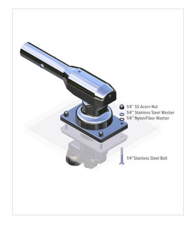
Deluxe Base. We recommend using nylon/fiber washers, stainless steel washers, and stainless steel acorn nuts to complete the mounting arrangement. Clean up excess sealant with acetone if necessary (DO NOT USE alcohol-based cleaners).
